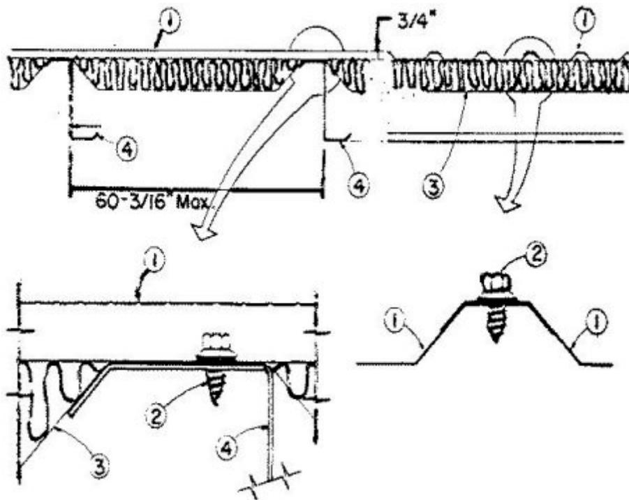
**1. Metal Roof-Deck Panels\*** No. 26 MSG min gauge coated steel. Panels continuous over two or more spans. End laps to occur over purlins with panels overlapped 6 in. with lap centered over purlin web. A bead of sealant may be used at panel end and side laps.
