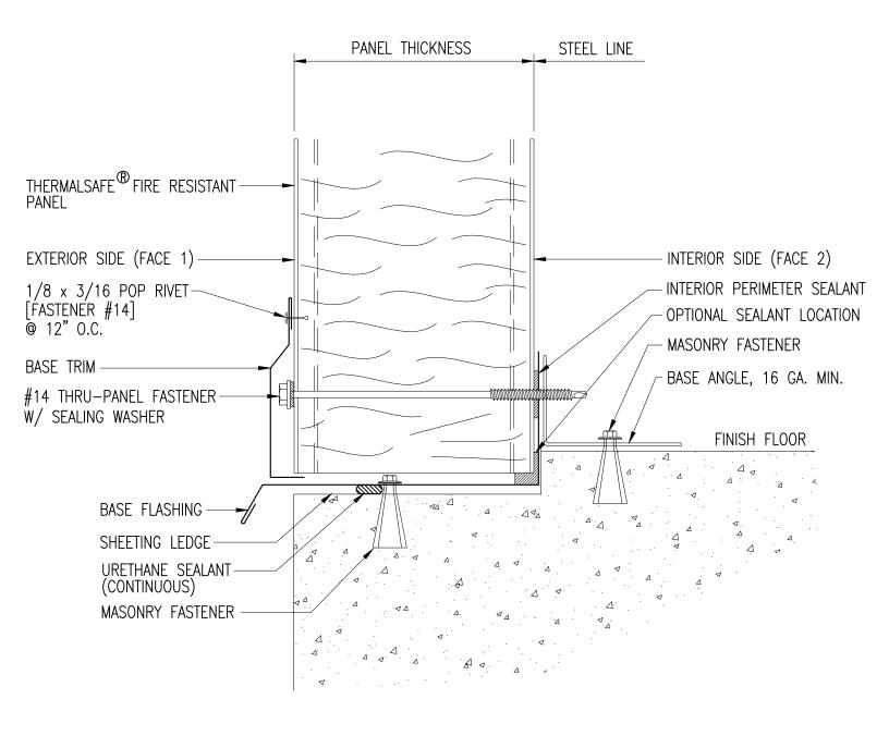
VERTICAL PANEL — BASE DETAIL (THRU-PANEL FASTENED)
