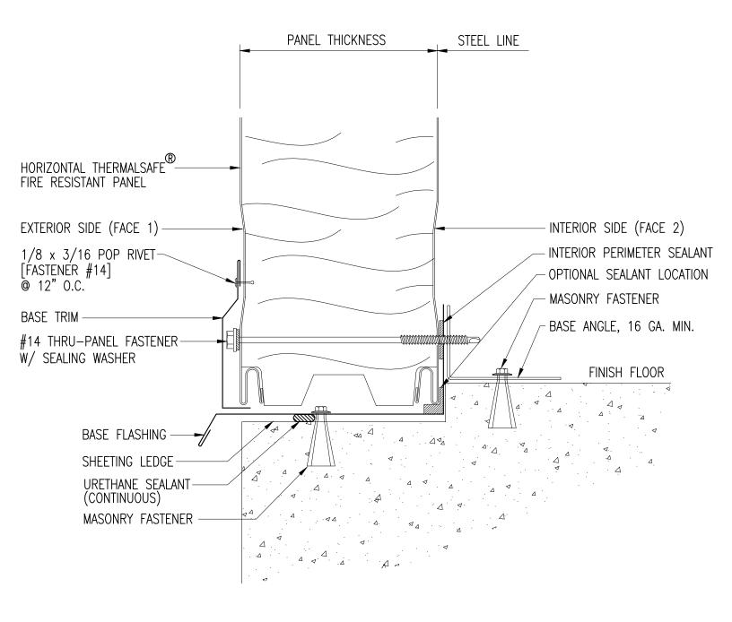
HORIZONTAL PANEL — BASE DETAIL (THRU-PANEL FASTENED)
