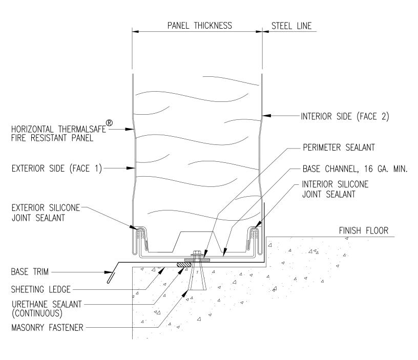
HORIZONTAL PANEL - BASE DETAIL (W/ BASE CHANNEL)
