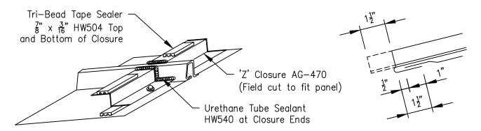
Field Notch Panel Legs 1 1/2" and Bend Pan to Form Open Hem Note: Panels With Minor Ribs Cannot be Hemmed
