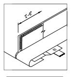
FIELD APPLY BEAD OF URETHANE SEALANT TO VERTICAL LEG OF PANEL BEFORE INSTALLING ADJACENT PANEL
