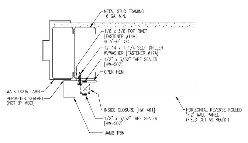
NOTE: MBCI RECOMMENDS THAT A REVERSE ROLLED 7.2 PANEL BE USED IN HORIZONTAL APPLICATIONS SO THAT THE LAP FASTENERS CAN BE INSTALLED IN THE LOW RIBS.
