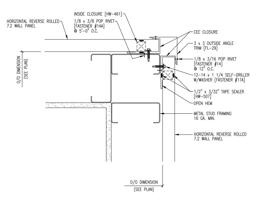
NOTE: MBCI RECOMMENDS THAT A REVERSE ROLLED 7.2 PANEL BE USED IN HORIZONTAL APPLICATIONS SO THAT THE LAP FASTENERS CAN BE INSTALLED IN THE LOW RIBS.
