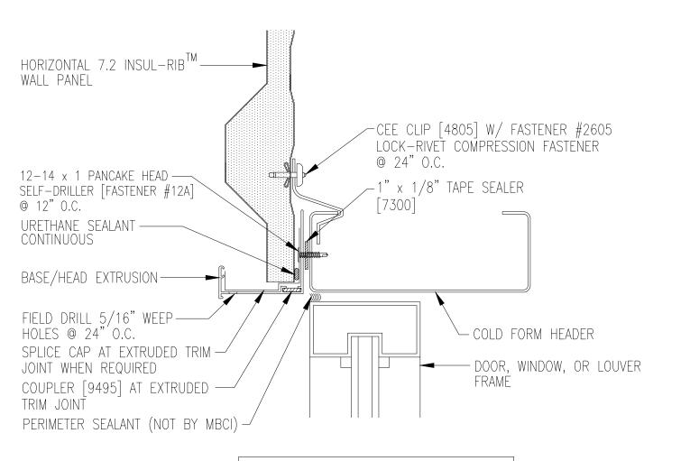
NOTE: THIS DETAIL CAN ONLY BE USED WITH 3" & 4" THICK PANELS
