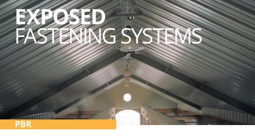
The PBR panel is commonly used for a wide variety of architectural, agricultural, commercial and industrial applications. PBR is a structural panel and an exposed fastener panel that can be used for both roof and wall applications. The minimum roof slope for PBR is ½:12.
